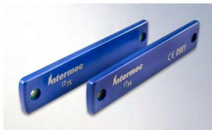
These ruggedised, metal-mount passive UHF tags, were selected as the appropriate tag type for permanent fixture on returnable assets for the job, after UMD's RFID testing and Proof-of-Concept stage was completed.
