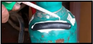
Apply the Adhesive_Paint to the bottom of the part, as well as an over-coat to the part
