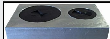
This perspective shows the tags mounted flush with the surface of the block.
