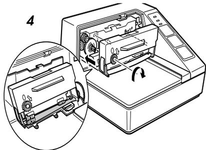
8. Push firmly on the right side and then the left side of the ribbon cartridge until each side clicks into place.
